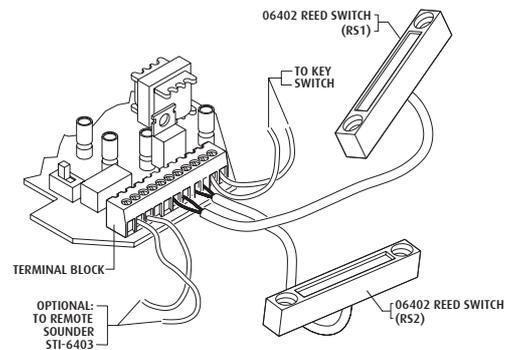
VIEW SHOWING INSTALLATION OF ADDITIONAL REED SWITCH 06402
