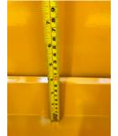
Some shelves are folded or are perforated with holes, so won't perform as a spill tray for smaller spills.
